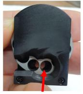
After rotating to the left side until a hole is stopped half by front cover, and then Insert a pellet into the hole on the lower left.
