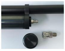
Do not use any other type of adapter other than the one supplied with the rifle. Slowly fill the rifle to a MAXIMUM of 230 bar (approximately 3,330 psi) pressure.
