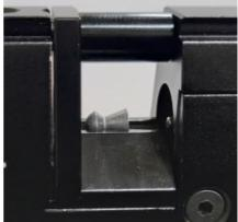
Put the tray on a gun like magazine after pulling rear bolt and put pellet on tray
